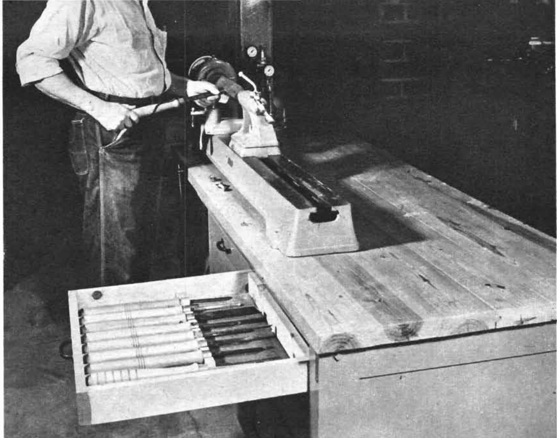
SLIDE-THROUGH DRAWERS can be opened from either side. Note dividing partition, built-in tool rack.
