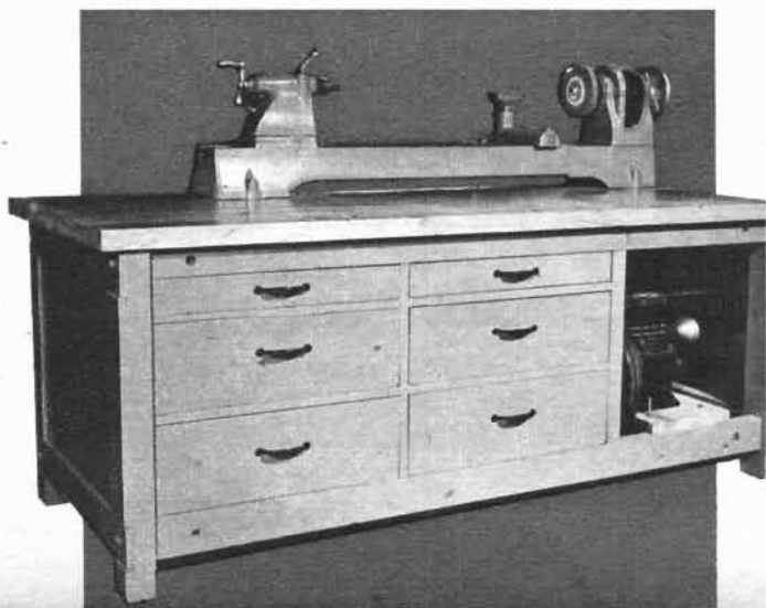
REAR VIEW of lathe bench shows the ample space available for the compressor mounted behind motor.
