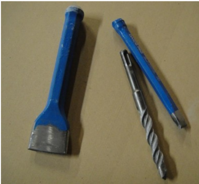
I don't mind buying cheap tools if they're going to be heavily abused. These concrete cold chisels have been reground several times, but they work well for how I use them.
