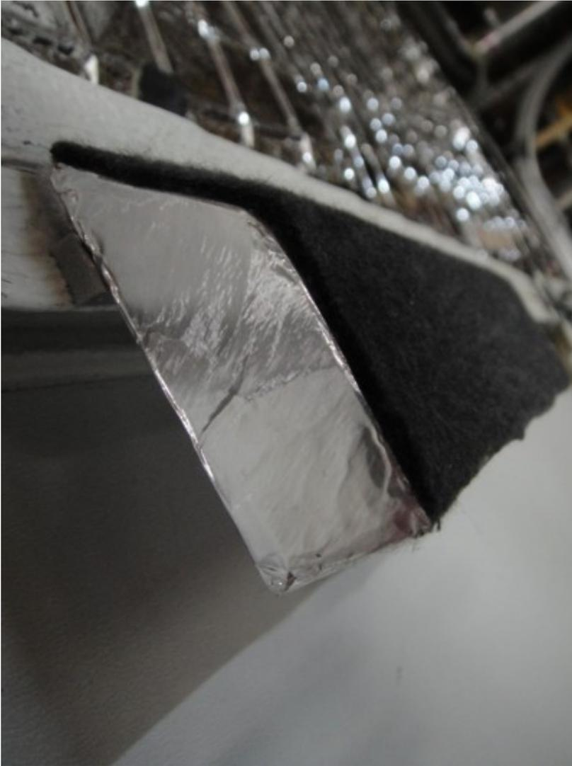
This is a mock-up I did for the panel construction. It's basically a 1" polyisocyanurate foil-faced foam sheet, with foil tape over the edges, with fleece (or felt) secured with spray adhesive, and the decorative fabric overlaid on top of it all.
