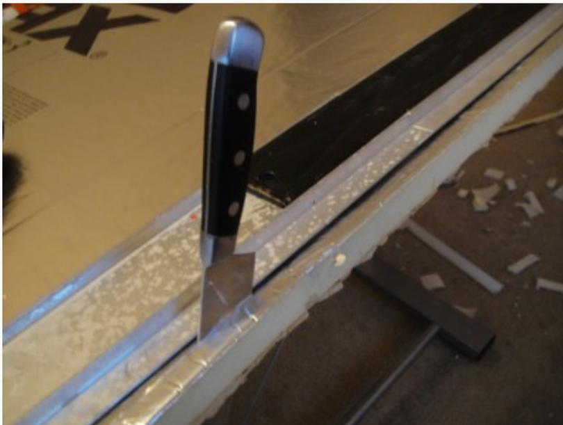
I use a cheese knife to cut these because it has small divets in the side of the blade that prevent it from sticking to the cheese (and in this case foam); works great and I do run it through a knife sharpener every so often.
