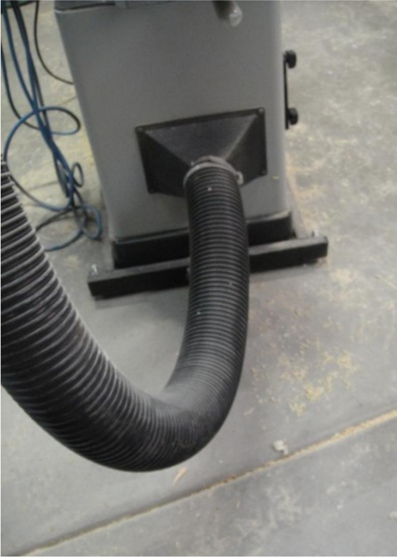
The Jointer I have comes with a 4" dust port but I find that it clogs with shavings. Plus, it's not getting close enough to the recommended CFM because of the higher static pressure the smaller diameter flex hose has.
