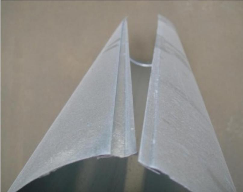
Snap-lock ductwork is easy to work with, including cutting. All you have to do is crimp one end, connect to the right fittings with sheet metal screws, and seal the seams with duct mastic.
