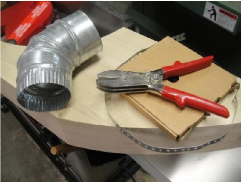
These crimpers allow you to fit the ducts together; just remember to point the crimped end toward the airflow.
